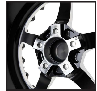
Fronts & Rears Feature Recessed Bolt Pads for Weight Reduction.
